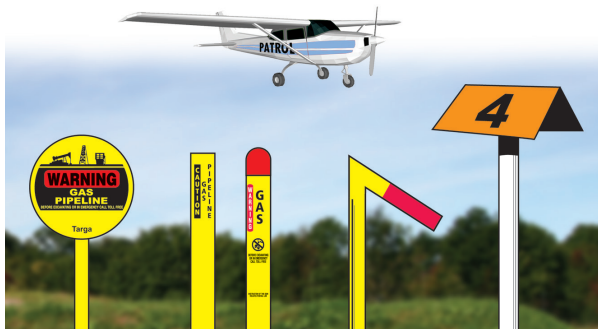
Located near roads, railroads and along pipeline right-of-ways Painted metal or plastic posts Pipeline casing vent Marker for pipeline patrol plane
